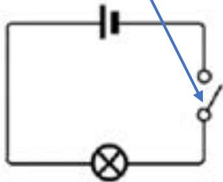
This breaks the circuit so it is not complete and electricity cannot flow. The bulb will turn off.
