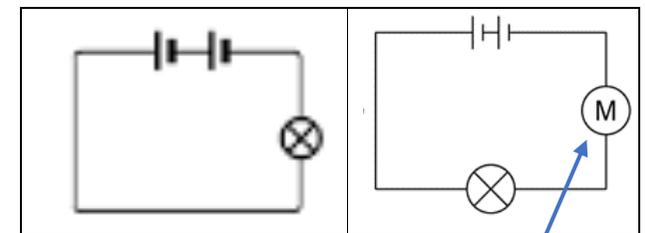
If we add a motor into a circuit with a single bulb, the bulb will be less bright.
