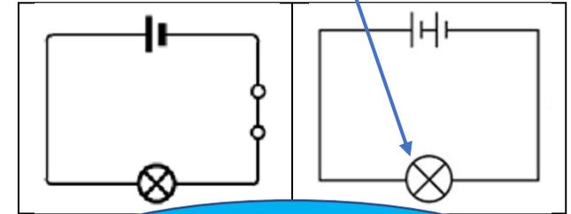
If you use a battery with a higher voltage, the bulb would also be brighter.
